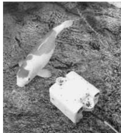
Figure 9. Laser scaling adapter installed on ROV – frontview (2). Figure 10. Laser scaling adapter installed on ROV – topview (2).
